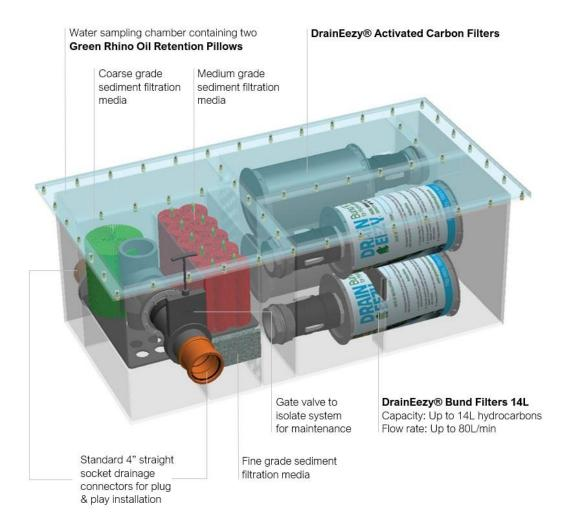
The Maxi system comprises a chamber which directs the flow of water through four levels of sediment and hydrocarbon filtration:
